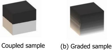
**Figure 1.** Schematic representations of the printed samples (SS: grey, HCl: black)
