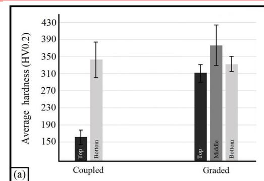
**Figure 5.** The average micro-hardness in different zones of 2 types of samples.
