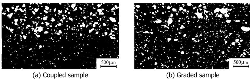
**Figure 2.** Optical microscope images taken from the cross section of two types of prints.
