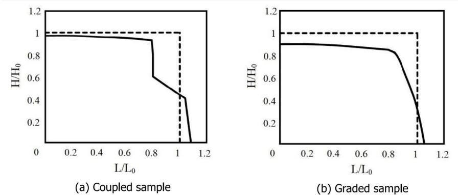
**Figure 3.** The dimensional profile of samples.  $L/L_0$  and  $H/H_0$  are the sintered/green ratios ( $H_0 = 9.82 \text{ mm}$  and  $L_0 = 5.28 \text{ mm}$ ).
