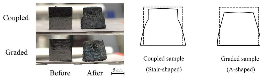
**Figure 4.** Images of green (before) and sintered (after), and distortion mode of samples.
